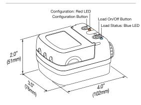
LMPL-101 Plug Load Room Controllers include a 1/2" (12.7mm) threaded nipple and locking ring.
